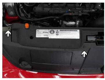
1. Remove the four (4) push pins from the top edge of the radiator cover. There are two (2) on each side. Then remove cover from vehicle.
