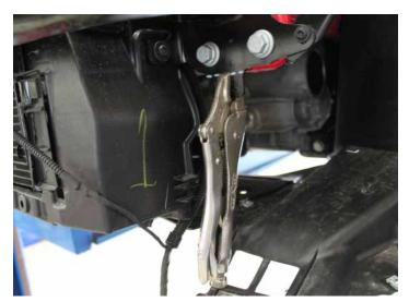
11. Remove the tab the horn was attached to flush with the body, either by bending back and forth with vise-grips as shown or using a reciprocating saw. Repeat on other side of vehicle. **WARNING**: If using a reciprocating saw be aware of the fluid reservoir on the passenger side when cutting.
