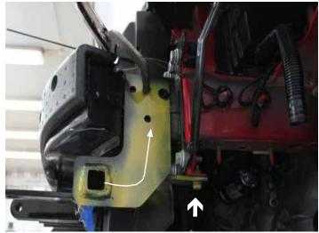
12. Rotate the baseplate from 90 degrees into place, attach at the bottom with a 8MM-1.25 x 30MM bolt, 8MM flat and lock washer. Level and clamp the baseplate. Drill the three (3) holes thru the frame using a 13/32" drill bit. Repeat on other side of vehicle.
