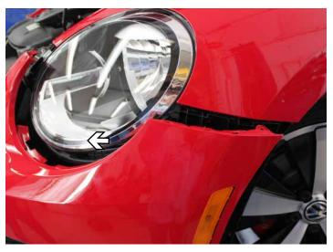
When removing front fascia, pull straight out and unhook both the side marker and running light wiring on both sides of vehicle.
