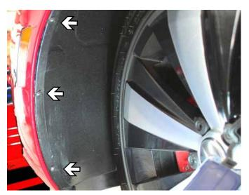
3. In the wheel well, use a T25 Torx to remove the three (3) screws. Do this to both sides of the vehicle.
