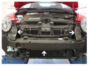
8. Remove the three (3) foam fascia support pieces. DO NOT discard these will be reinstalled.
